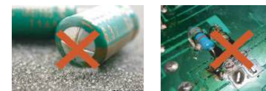
capacitor bulge and leakage
